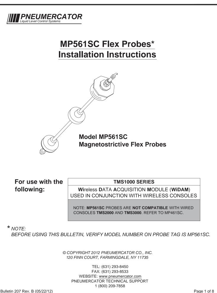
**PRODUCT DESCRIPTION:** MP561SC level gauging probes utilize proven magnetostrictive technology for accuracy and reliability. Probes are supplied with (1) product float for product level gauging and optionally (1) interface float for bottom water gauging. Additionally the probe contains either(1) or (5) thermistors for temperature measurement.
