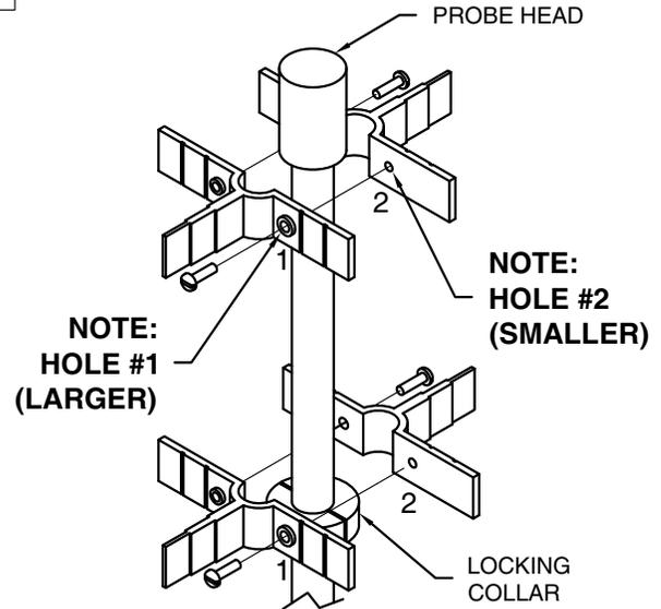
**2** Verify that the bottom of the locking collar is located 8" from the top of the probe head and confirm that collar is secured.
