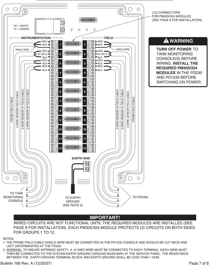
**MODULE INSTALLATION:** Align cutout with polarizing key for correct installation of module as shown below. In addition, the "FIELD" side of the module must be on the same side as the "FIELD" wording on the circuit boards for PD230 and PD1230.
