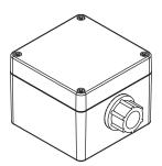
**PD1230 - 3x12 CHANNEL LIGHTNING SURGE PROTECTOR:** Model PD1230 provides protection for up to (36) circuits when (12) PM305 or PM324 modules are installed. PD1230s are generally installed as close as practical to a tank monitoring console such as Pneumercator E, LDE or TMS series.
