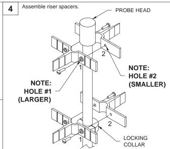
NOTE: AT THIS POINT MODEL MP452S/MP552S ASSEMBLY IS COMPLETE. PROCEED TO STEP 5 TO COMPLETE ASSEMBLY FOR ALL OTHER MODELS.
